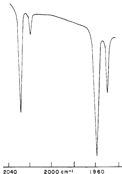
Fig. 3.—The \nu_3 band of \text{BO}_2^- in KBr matrix at 25^\circ . Boron isotopes in natural abundance.
